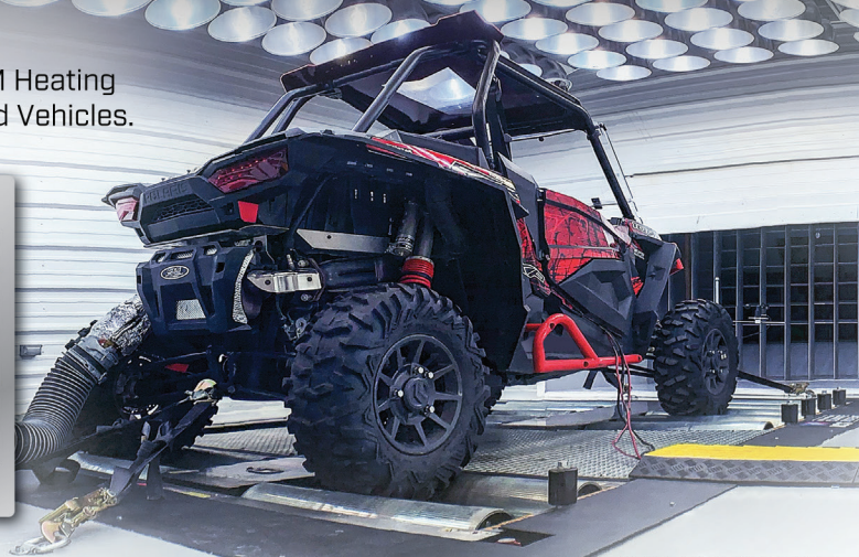
Photo: ICS Climate Tunnel dedicated to Off-Road Vehicle Testing
